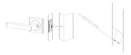
8.A.4: cut the marked area out with a depth of 3/32" that lipstrike is flush
